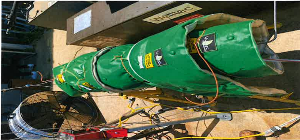
Figure 9: WFV with the conductors and isolation jackets for high temperatures
