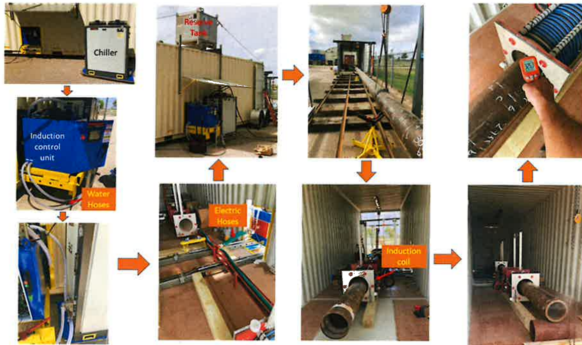
Figure 5: Full-scale set-up at The University of Oklahoma
